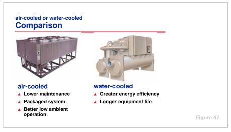
Water-cooled chillers are generally more energy efficient. The efficiency advantage of a water-cooled chiller, however, is much less when the additional cooling tower and condenser pump energy costs are considered. Additionally, this efficiency advantage may lessen at part-load conditions since the dry bulb temperature tends to drop faster than the wet bulb temperature and the aircooled chiller benefits from greater condenser relief.
